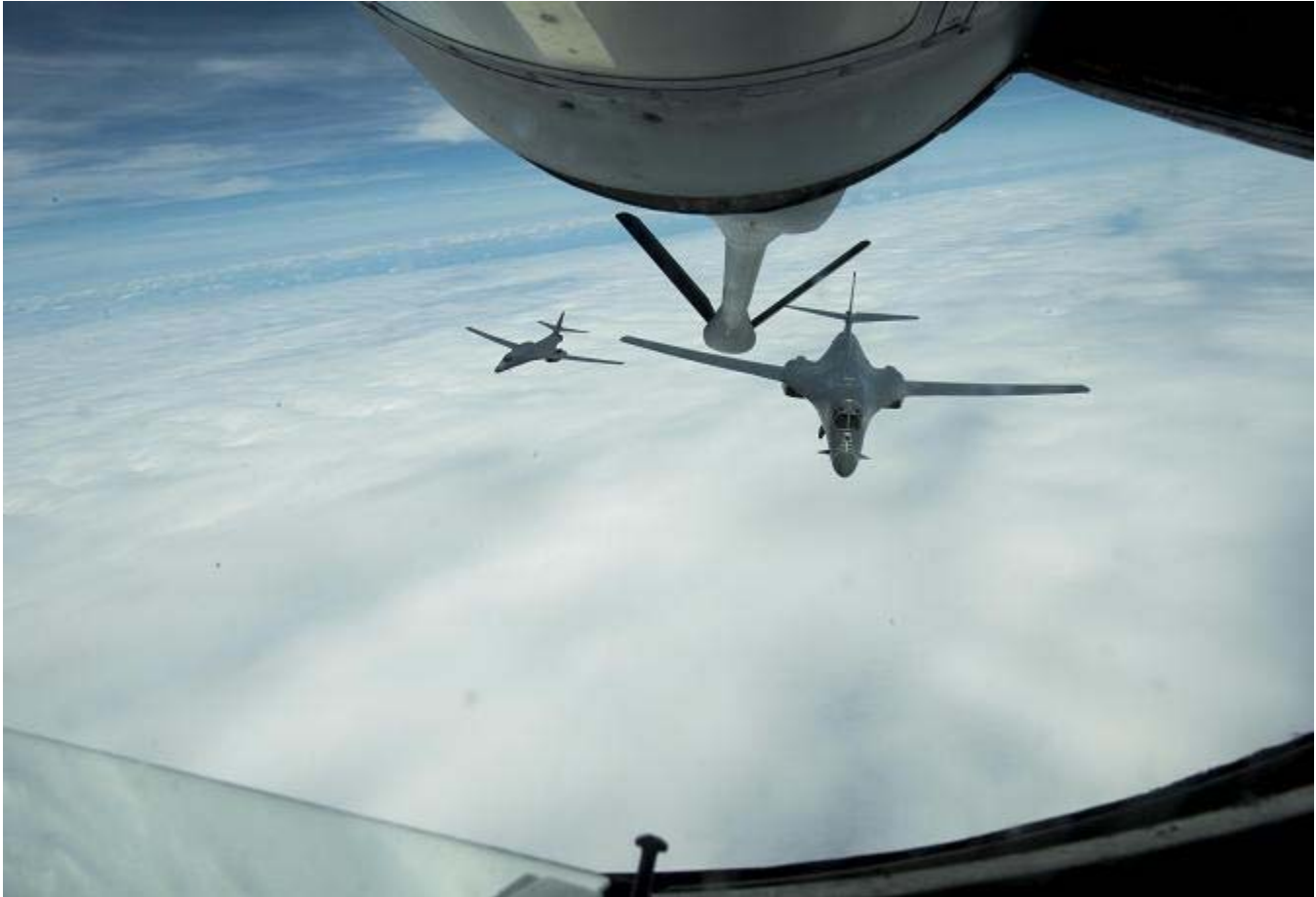
U.S. Air Force B-1B Lancers assigned to the 9th Expeditionary Bomb Squadron prepare to depart after receiving an in-flight refuel from a KC-135 Stratotanker during Cope North 2017, Feb. 16, 2017. The exercise included 22 total flying units and more than 1,700 personnel from three countries. U.S. Air Force photo by Senior Airman Keith James.
