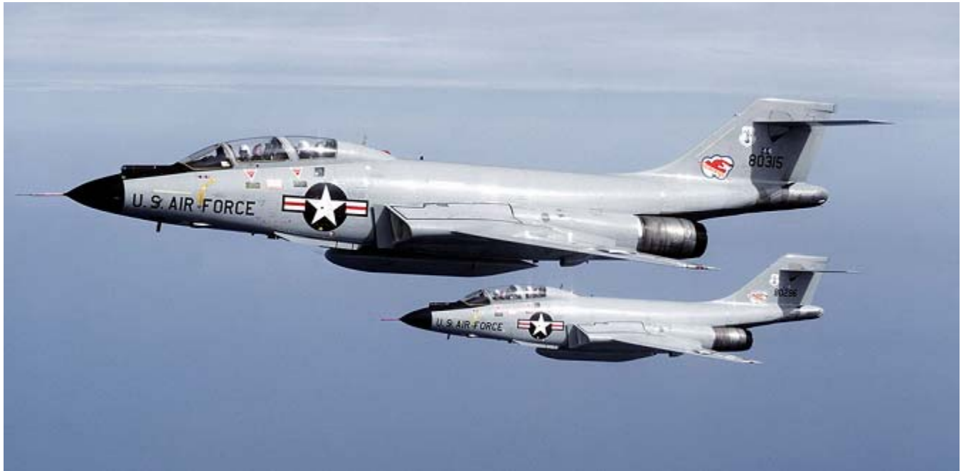
The F-101B was initially designed by McDonnell Aircraft as a long-range bomber escort (known as a penetration fighter) for the Strategic Air Command. The Voodoo was instead developed as a nuclear-armed fighter-bomber for the Tactical Air Command, and as a photo reconnaissance aircraft based on the same airframe. USAF photograph.
